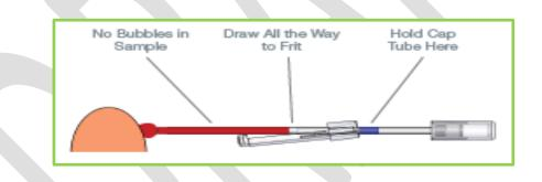
**6.5.3** To fit the adaptor over the end of capillary tube, push tube into adaptor until secured.
