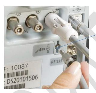
Using the nitric delivery line from the back of the head, unclip this and press on to the purge port. An audible noise (hissing) should be heard.
