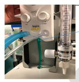
Disposable oxygen tubing to be cut to around 2m length (length of incubator). One side to be connected to rPAP.
