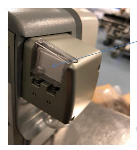
Insert water separation cartridge into slot at side of monitor (rear end).
