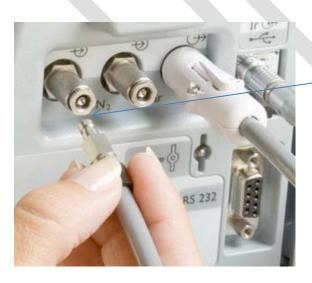
When the regulator pressure gauge reads zero, remove the regulator hose from the purge port and connect it to the INOMAX gas inlet ready for delivery.
