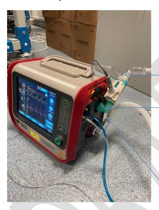
Connect Hamilton neonatal tubing direct to injector module. The arrow must point the way of the gasses will flow (upwards to inspiratory limb)
