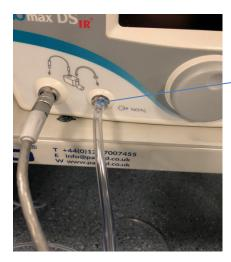
Connect NO injector tube to port on INOmax machine.
