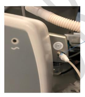
Connect gas sample line to connector at side of INOmax head.
