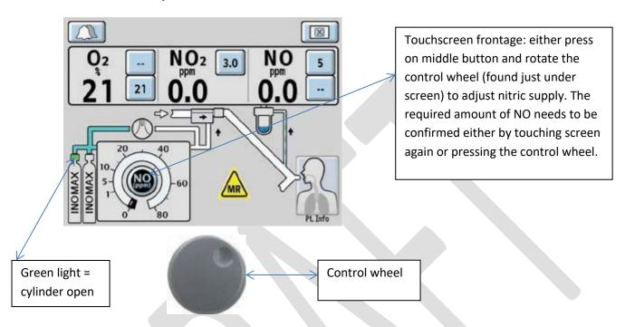
This will then allow the correct amount of NO to be delivered to the patient if following the set up and using the touchscreen delivery display. This can be adjusted as required.
