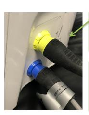
Plug both heater cables into the side of the humidifier (blue to blue, yellow to yellow).
